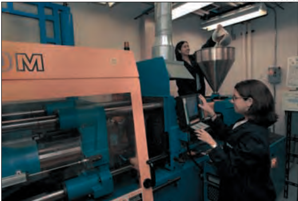
Angela Harris and Ellen Lee of the Biomaterials Group injection molding wheat straw reinforced polypropylene specimens for testing.
