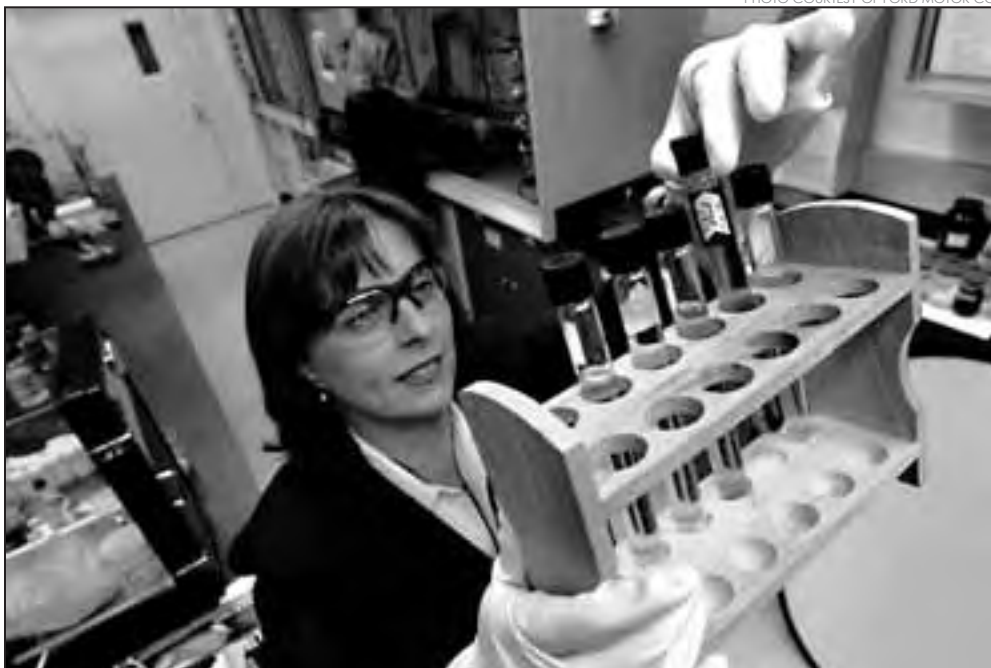
Debbie Mielewski examines soy-based polyol samples. The soy polyol is similar in structure to that produced from petroleum.
