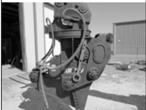
NEW Cat MP15 - 4,500 lb multi-processor with shear jaws and 360 rotation. Bracket for Cat 320 stick. $59,500
