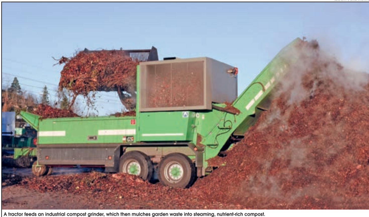
A tractor feeds an industrial compost grinder, which then mulches garden waste into steaming, nutrient-rich compost.
