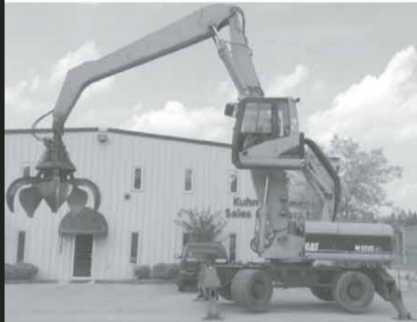
2006 Cat M322C MH - Hydraulic cab, A/C, 41 ft. reach MH boom & stick, gen set, Cat grapple, and solid tires. Call For Price!
