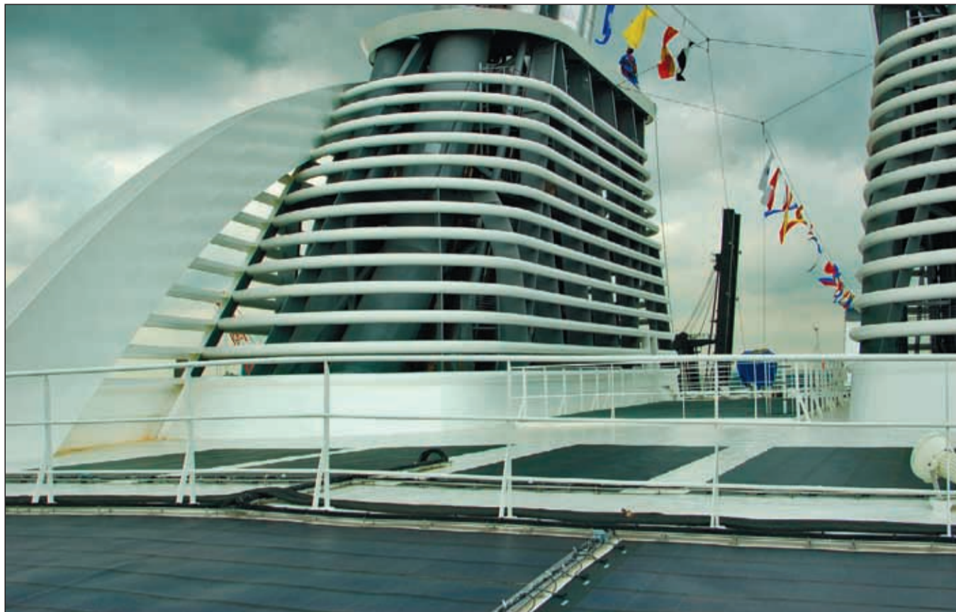
Photovoltaics strong enough to walk on and durable enough to be at sea were installed on the Allure of the Seas cruise ship.
