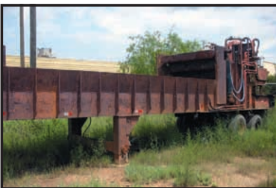
AL-JON CAR CRUSHER WITH AUTOMATION
