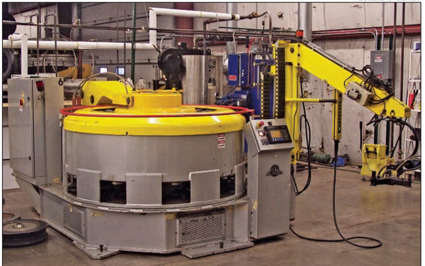
A CIMA tire press produces 315/75R16, 315/70R17 and 37x12.50R16.5 tires in the Guard Dog tread pattern. The tires are cured in the press at temperatures of over 300 degrees and at pressures of approximately 150 psi.
