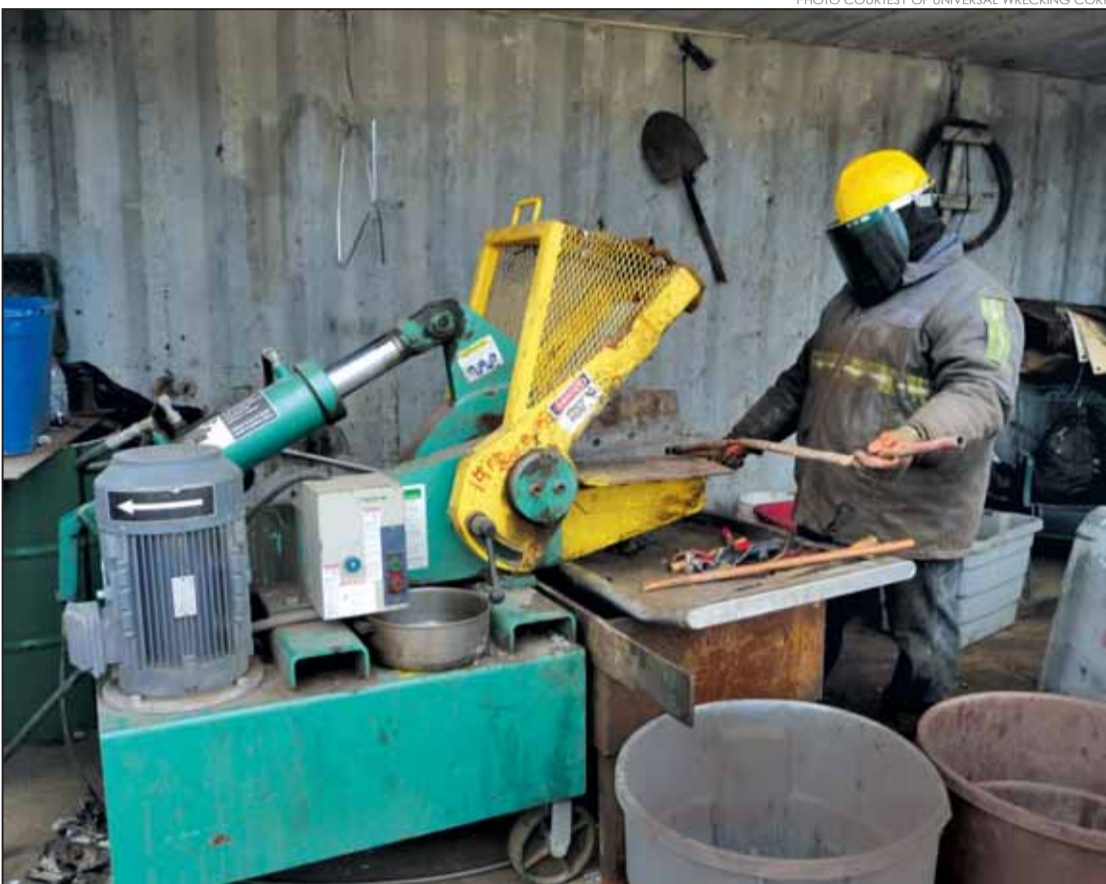
Scrap copper hydraulic cutter area at Universal Wrecking, Bayville, New Jersey. Worker wearing proper PPE (face shield, work gloves and long sleeve jacket). Fire extinguisher is nearby.
