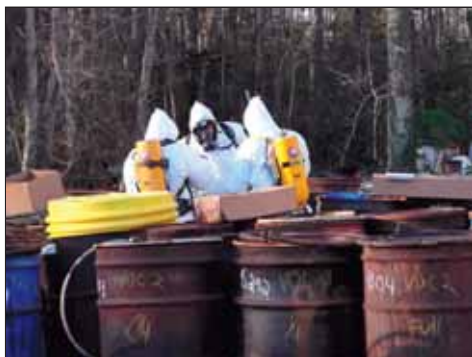
Sampling teams use supplied air for breathing and monitor the ambient environment with multi-gas meters at the Superior Barrel & Drum Site. PHOTO COURTESY OF US EPA
