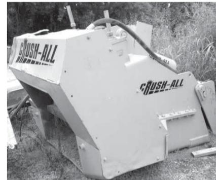
Used as an attachment on excavators. Crush concrete, concrete with rebar, rock, block, brick, asphalt, asphalt shingles, many other breakable products. Weight: 10,000 lbs.
