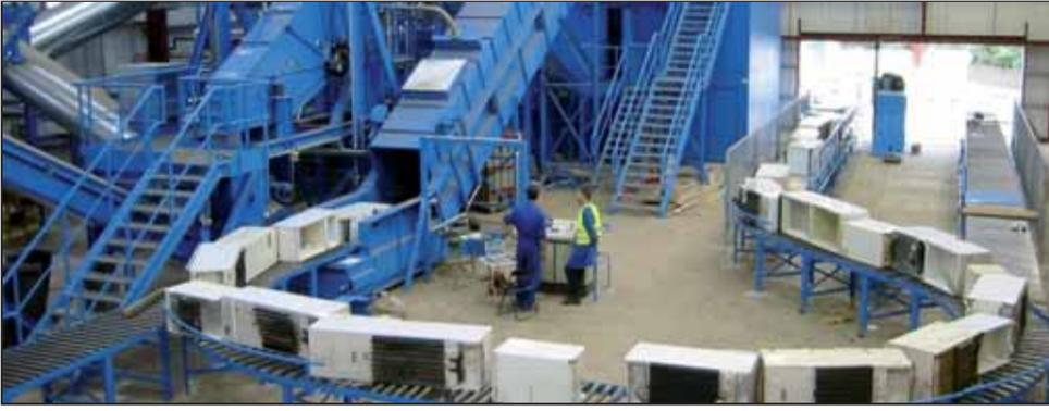
In recycling of refrigerators, the main goal is to generate clean fractions of aluminum, copper, iron, and plastics so that these can be sold on the secondary raw materials market. One of the biggest challenges is to filter out the harmful CFCs, which adhere mainly to the polyurethane foam insulation.
