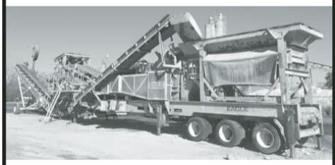
2012 Eagle Ultramax 1200-25 CC - 4,100 hours, Impact Crusher, closed circuit, 2 deck screen, vibrating primary screen, magnetic separator, stacking conveyor and scale. Call for price!
