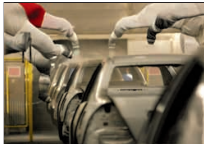
Water-borne coatings are applied to cars and light trucks at the new paint line that opened in 2006 at Honda of America Manufacturing's auto plant in Marysville, Ohio. The line significantly reduces chemical emissions and contributed toward earning the Energy Star award.
