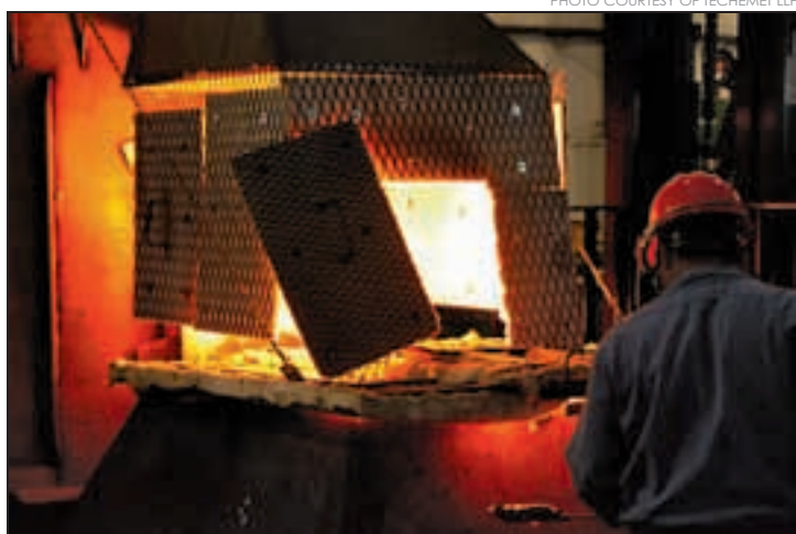
Slag tapping at Techemet from submerged electric arc furnace removes impurities to refine platinum group metals from ceramic catalyst materials.
