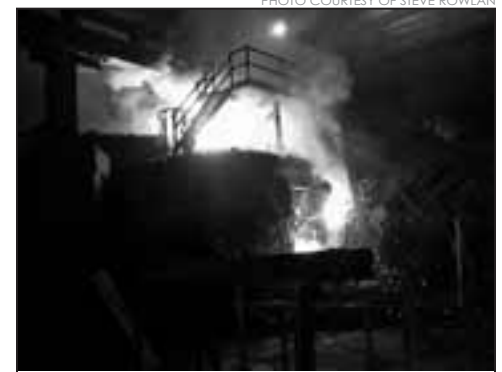
An electric arc furnace recycling tons of scrap metal into new high quality steel.
