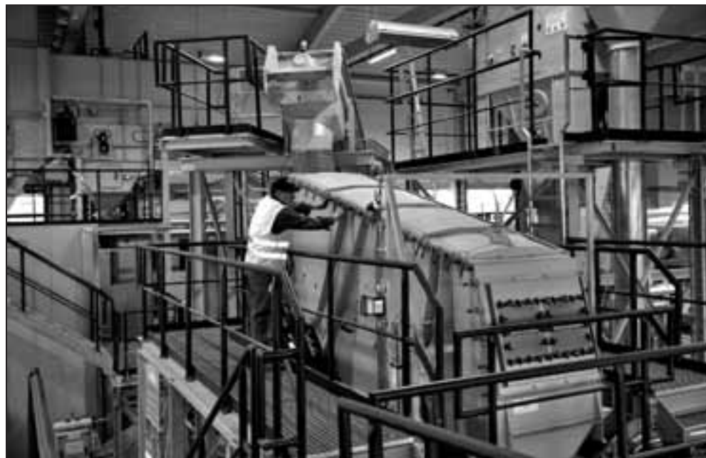
A device at the screening station for PUR foam separates the fine ground PUR foam from metal, aluminum and plastic fractions.
