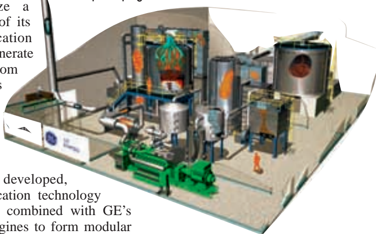
An illustration of Nexterra's 2 MWe commercial demonstration plant featuring a GE Jenbacher engine that will be built in Phase 2 of the biomass power program.
