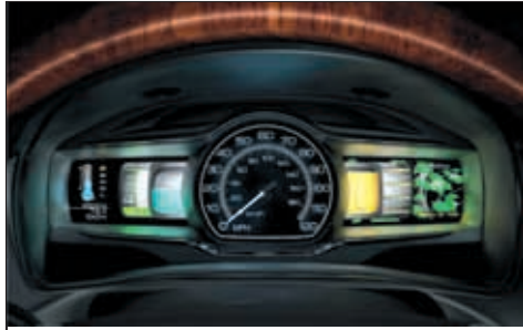
SmartGauge™ with EcoGuide is an instrument cluster that coaches hybrid owners on how to maximize their fuel efficiency.
