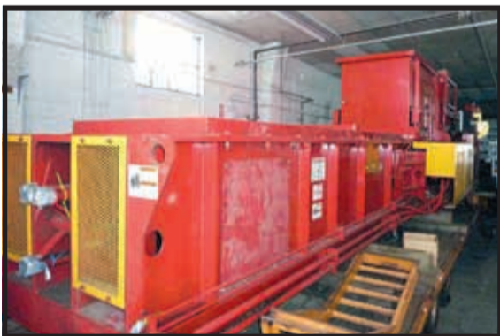
2007 MARATHON MODEL: 2R 190N (2) 30 hp motors, main cylinder: 9". Feed Opening: 40" x 70". Bale separation door. Used under 6 months. $205,000
