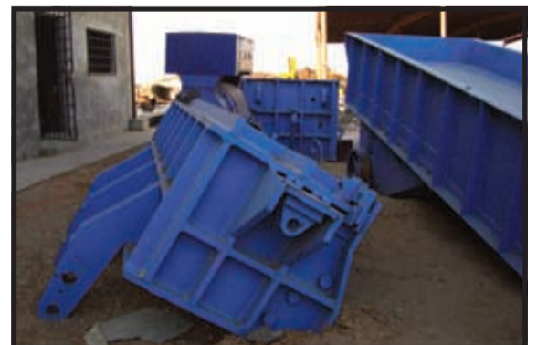
JEFFERY 62 x 90 HAMMERMILL SHREDDER REBUILT. 800 h.p. electric motor (accepts up to a 2,000 h.p. motor) and an extra base, reversible hammers and oscillator table. Also a pin puller, slope feed table, drive sheaves, tilt cylinders, bearings and eddy system. $450,000
