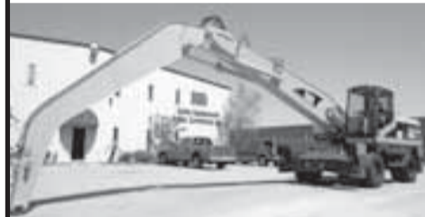
2000 Cat M320 MH - 38 ft MH arrangement, standard cab, NEW 12 kw gen set, and "like new" solid tires.
