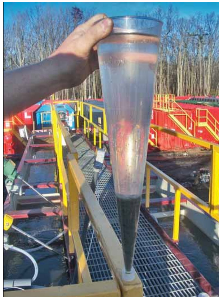
Treatment is effective enough that recycled frack water can be re-used over and over for future frack jobs.
