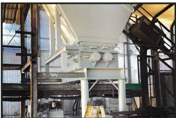
SSI 1400-E SHREDDER 150 hp, 30 x 30 opening, new 2.25" knives, hydraulic HydroStar motor. $65,000
