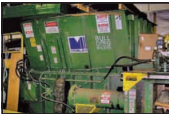
1996 MOSLEY BULLDOG BALER 200 h.p., 12" main cylinder, bale release. Reconditioned with 90 day warranty $195,000
