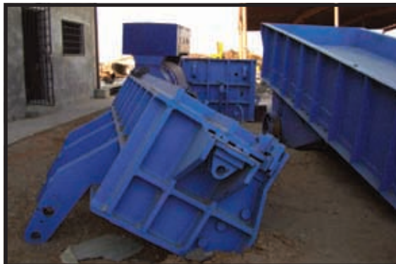
JEFFERY 62 x 90 HAMMERMILL SHREDDER REBUILT. 800 h.p. electric motor (accepts up to a 2,000 h.p. motor) and an extra base, reversible hammers and oscillator table. Also a pin puller, slope feed table, drive sheaves, tilt cylinders, bearings and eddy system. $450,000
