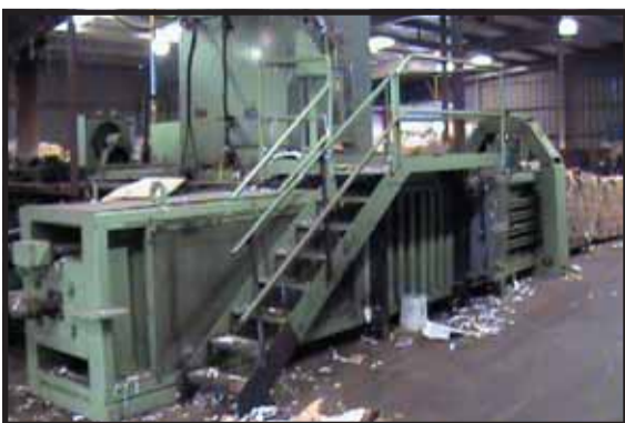
REBUILT EC 2 RAM BALER 150hp, 12 cylinder, PLC upgrade, soft start. Excellent for OCC, high grade paper, LDPE film, and shrink wrap. $120,000
