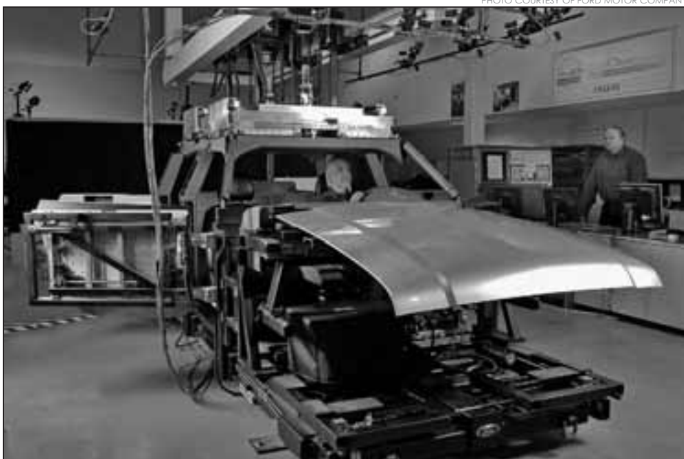
A Ford design laboratory where engineers, with the aid of lifesize parts and computers, can test chassis designs to maximize passenger comfort and ease of servicing and dismantling.
