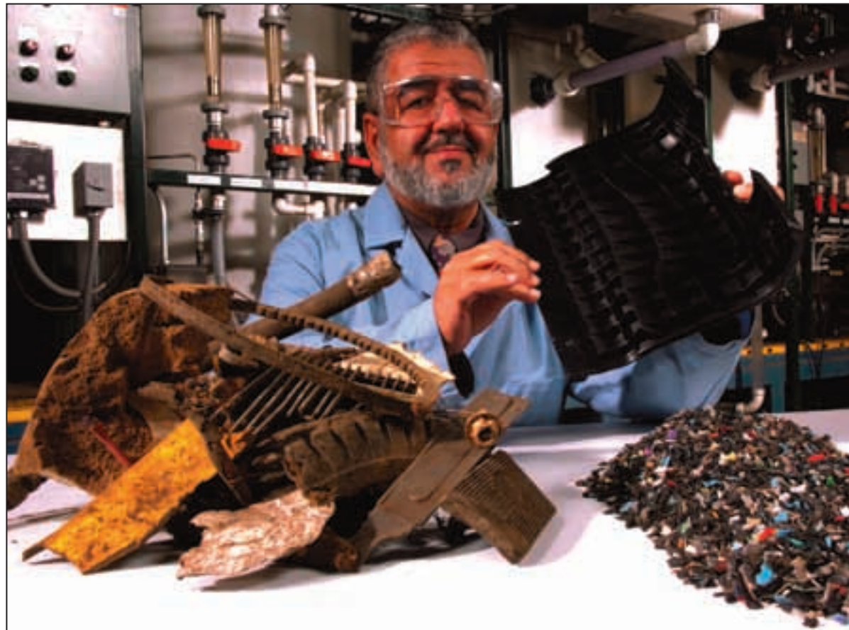
Bassam Jody, group leader of the energy systems division at the Argonne National Laboratory, displays plastics recovered from shredder residue by the Argonne Separation process and successfully tested for making auto parts.
