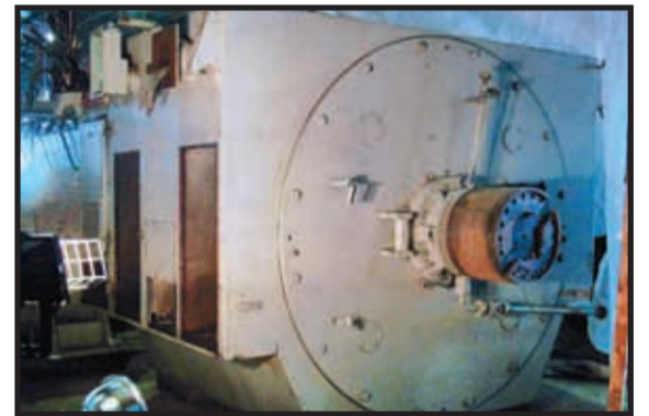
4,000 HP TOSHIBA REWOUND SHREDDER MOTOR
