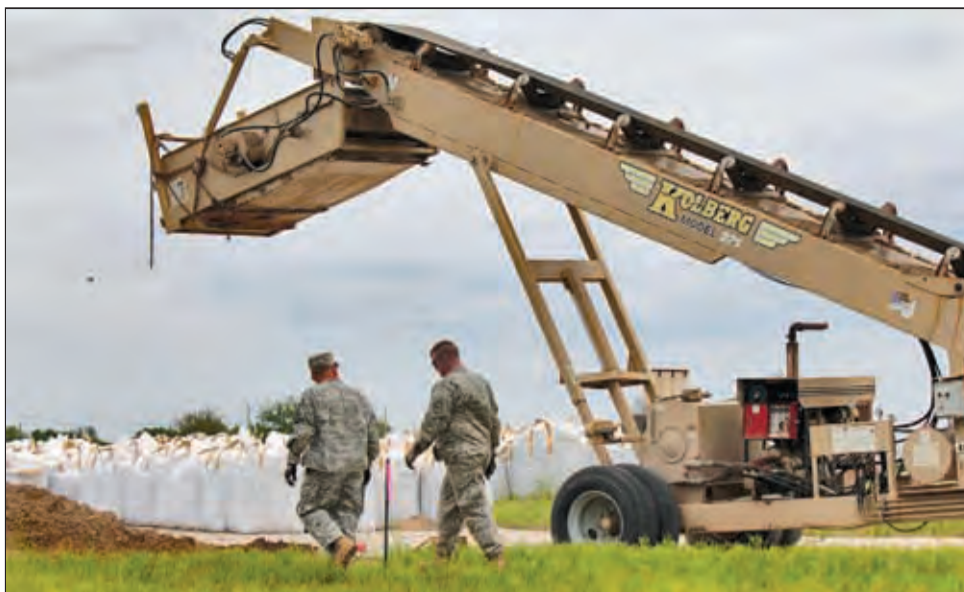
Service members from South Dakota's National Guard use a Series 271 Screening Plant, which was engineered and manufactured at KPI-JCI in Yankton, South Dakota, to fill sandbags during recent flood relief efforts in Dakota Dunes.
