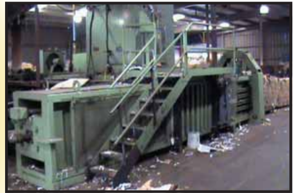
REBUILT EC 2 RAM BALER 150hp, 12 cylinder, PLC upgrade, soft start. Excellent for OCC, high grade paper, LDPE film, and shrink wrap. $120,000
