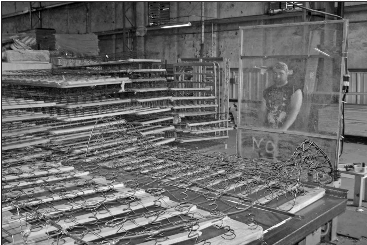
Unfortunately, mattresses are not easily processed by many common recycling machines and methods. Therefore, much of the tear down and separation of recyclable components must be done by hand.
