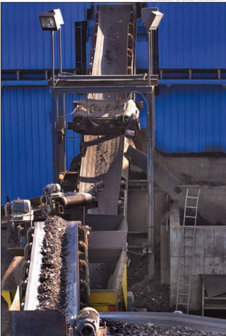
ASR en route to the eddy current separators at the Upstate Shredding plant in Owego, New York.
