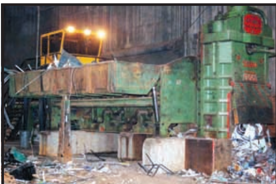
2005 SIERRA 700-TON SHEAR LOGGER BALER
