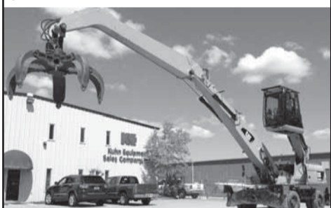
2010 Cat M322D MH - 3,800 hrs, hydraulic cab, A/C, 41 ft. MH boom & stick, outriggers, solid tires, camera, gen set, and grapple. $259,500
