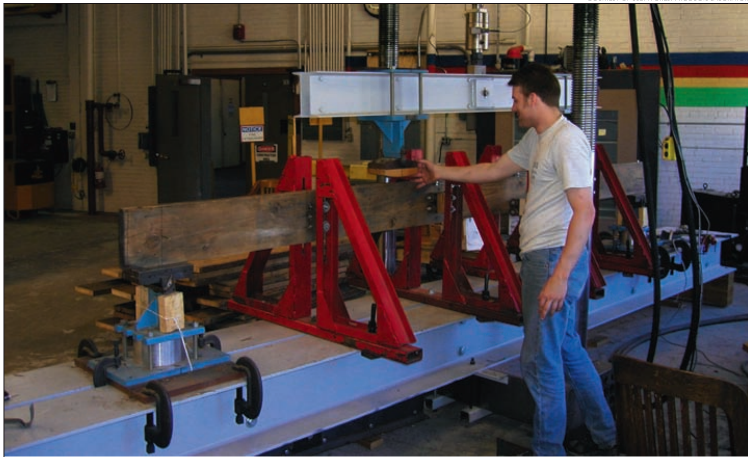
Reclaimed wood is put through stress testing to ascertain its suitability for use in other projects. Markets for recovered lumber are expected to grow as current grading standards are updated to include standards for recovered wood.
