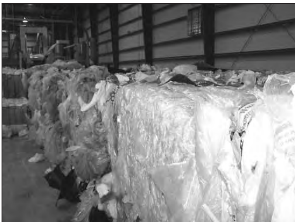
Multiple bales of plastic bags await shredding and further processing. The finished product may be used in the manufacture of new bags or other useful products.
