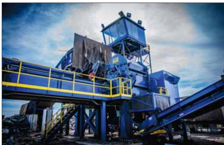
Wendt M6090 shredder with 2,500 hp motor is capable of shredding 3,000 to 8,000 tons per month.
