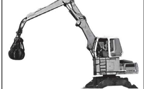
4' Elevated Cab, 10 KW Generator 36' Reach, Grapple 49,500 lb. Operating Weight
