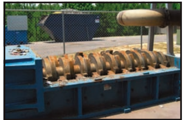
SHRED-PAX AZ 160 MATERIAL SHREDDER Motors and gear box refurbished 12/08. Double stacked and staggered hook knives. Includes support frame, feed hopper, hood and control panel. Opening 96" x 44" with (2) 75 h.p. motors $165,000
