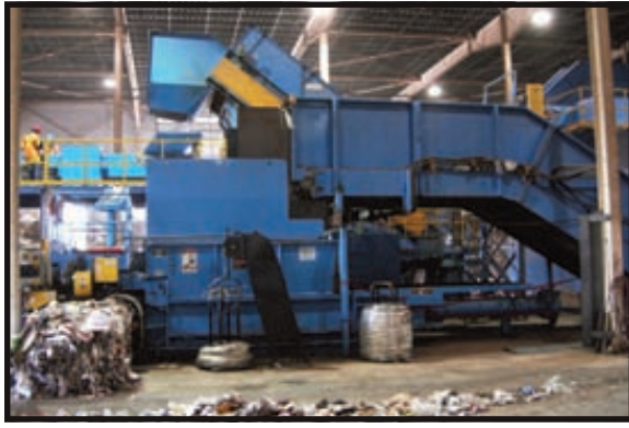
LOGEMANN 245A-1-AT BALER Left-hand stationary baler with extensive rebuilding and is ready to go. (2) 100 h.p. 480v with a new Accent Wire Tier, 12" main cylinder. Loaded on your truck. $195,000
