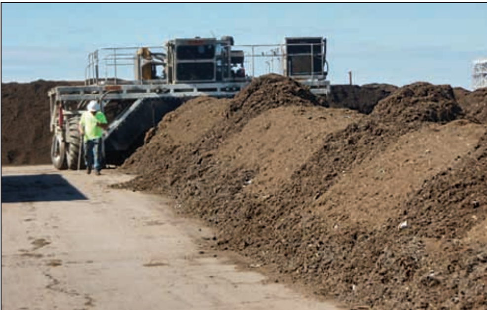
Agromin cleans and chops green waste before laying it out in composting rows.
