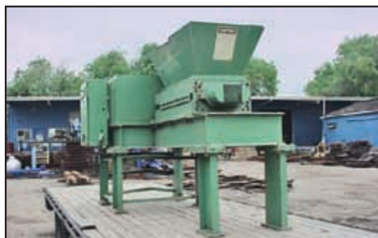
TRS KNIFE SHREDDER 40 x 22 40 h.p. motor and controls, stand. Six-month warranty. Great for non-ferrous, tires, plastic, etc. $65,000
