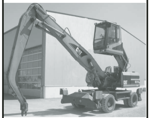
2002 Cat M318 MH - 35 ft reach, hydraulic cab, heat & A/C, gen set, 3/4 yd3 grapple, and solid tires. Call for Price!
