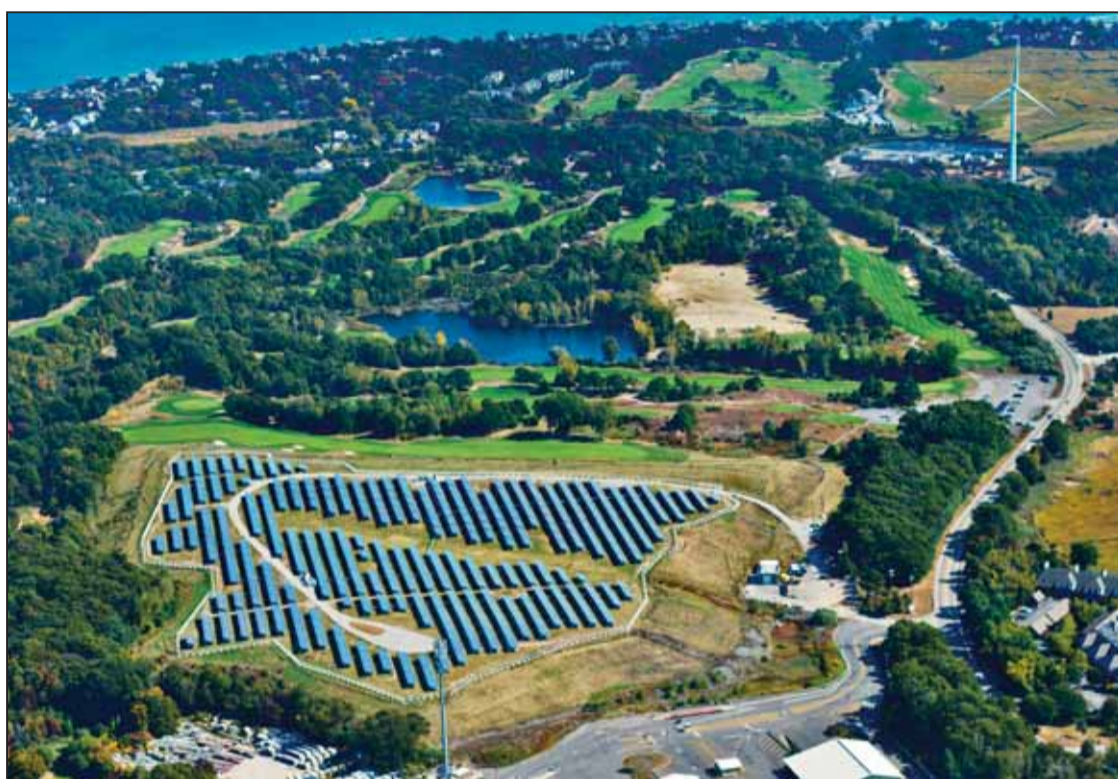
This solar project was constructed atop the Massachusetts town of Scituate's capped landfill, converting a dormant property into a valuable asset. When combined with the wind turbine output, the town will use 100 percent renewable energy to power all of the town's municipal facilities.
