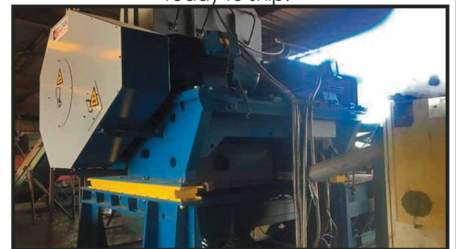
2014 Eldan Tire Rasper System. w/magnets, baghouse & deluge system.
