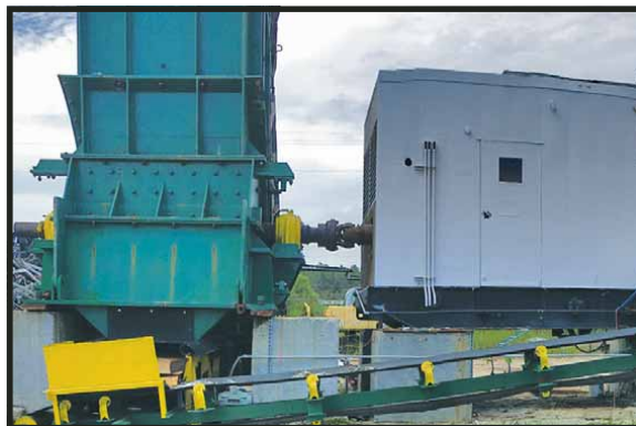
WILLIAMS 60 X 90 HAMMERMILL SHREDDER
