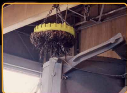
Production Scrap Handling Magnets 20" – 93" diameter
