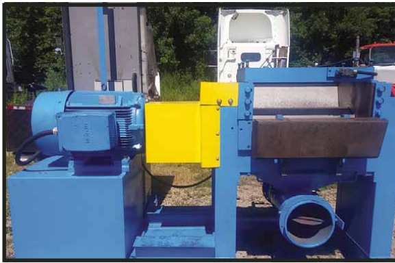
CUMBERLAND MODEL 30 TIRE GRANULATOR Recently rebuilt, 100 hp
