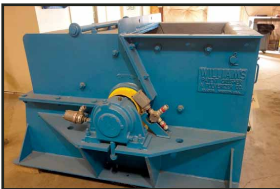
WILLIAMS 42 x 29 HAMMERMILL SHREDDER 250 HP motor, 50lb. hammers.
