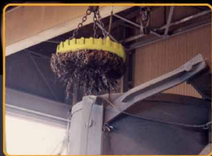
Production Scrap Handling Magnets 20" – 93" diameter
