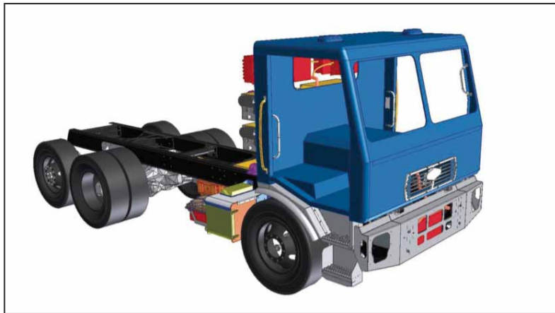
The Motiv All-Electric Powertrain, installed on the Sacramento electric refuse truck, transforms a chassis meant to be diesel powered to one with zero emission all electric drive, giving fleets an easier transition to a fossil fuel free future.
