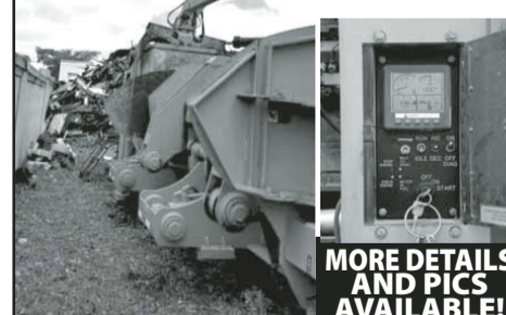
2011 Cat M322D MH - 5,205 hours, 37 ft. reach, heat and A/C, hydraulic cab, sorting stick, and NEW Cat G320B sorting grapple. Call for Price!
