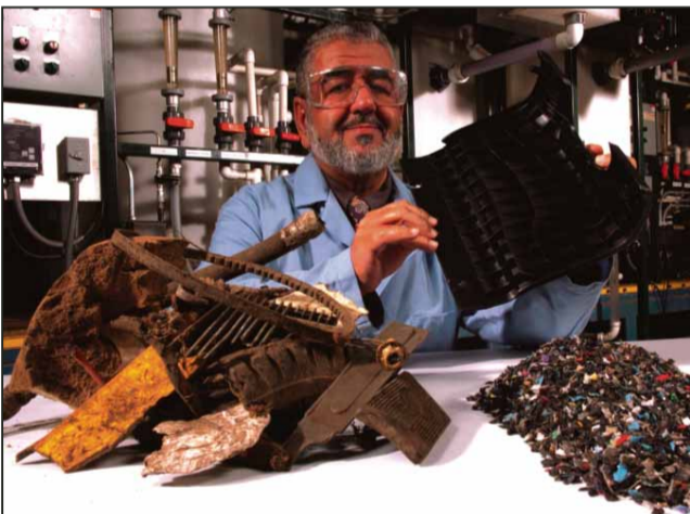
Bassam Jody, previous group leader of the energy systems division at the Argonne National Laboratory, displays plastics recovered from shredder residue by the Argonne Separation process and successfully tested for making auto parts.
