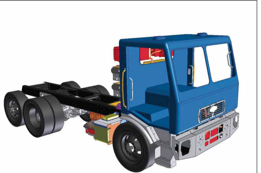
The Motiv All-Electric Powertrain, installed on the Sacramento electric refuse truck, transforms a chassis meant to be diesel powered to one with zero emission all electric drive, giving fleets an easier transition to a fossil fuel free future.
