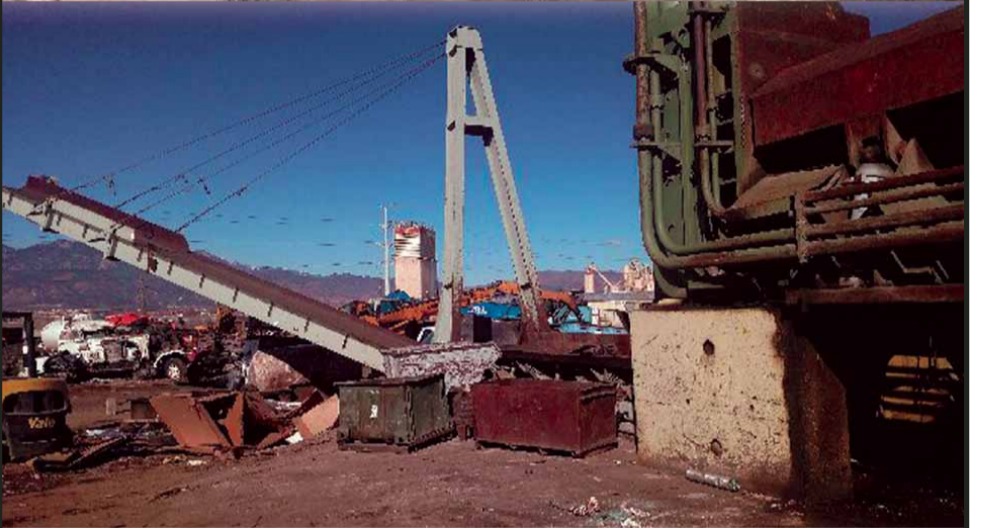
2005 Sierra 750T Shear. Includes a vibrating discharge conveyor and a stacking conveyor. $295,000
