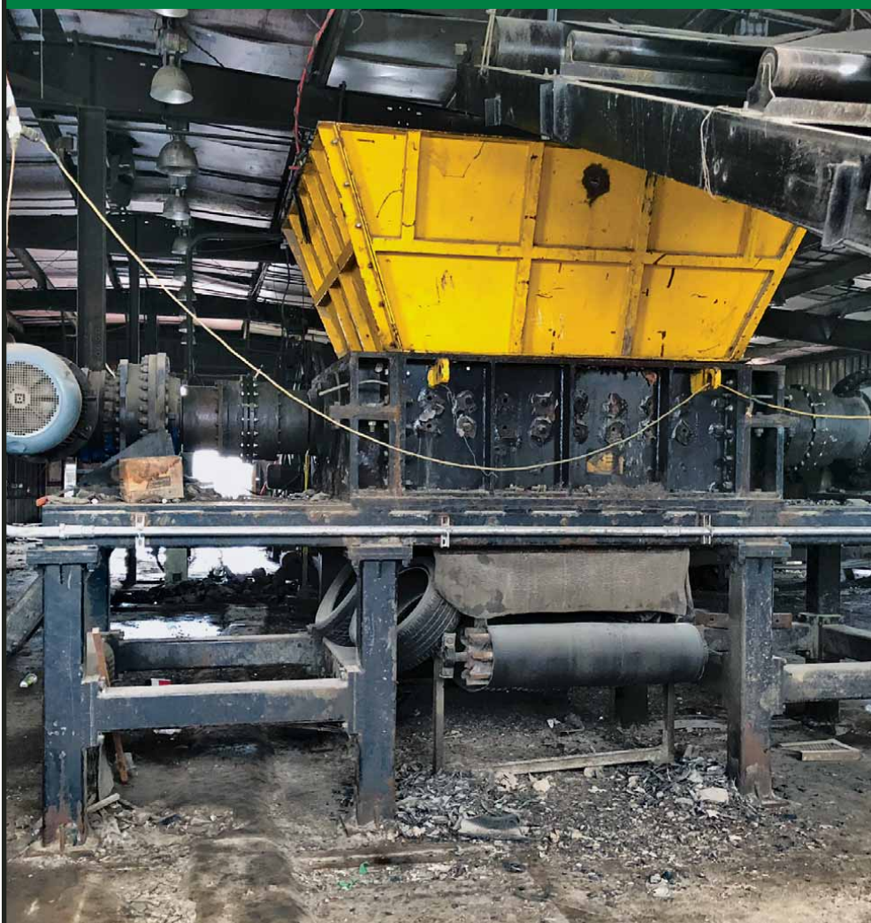
2009 E-3 Primary Tire Shredder. Shreds OTR tires with 3" bead. 2" double stacked knives. $145,000
