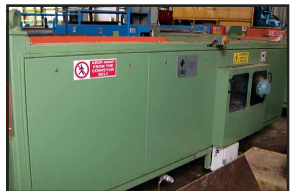
2012 SGM 40 FINES EDDY CURRENT SYSTEM
