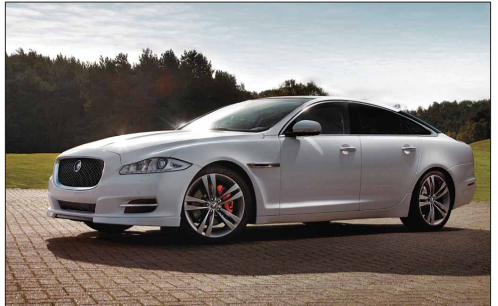
Featuring 75 percent aluminum in the Body-in-White, the aluminum-intensive vehicle sets a new standard for automotive aluminum lightweighting solutions in China.
