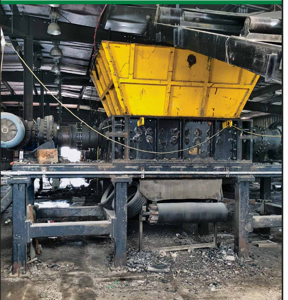
2009 3-E Primary Tire Shredder. Shreds OTR tires with 3" bead. 2" double stacked knives. $145,000
