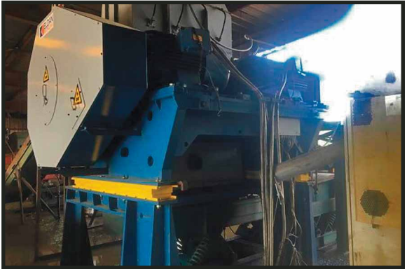
2014 ELDAN TIRE RASPER SYSTEM Includes magnets, baghouse and deluge system.
