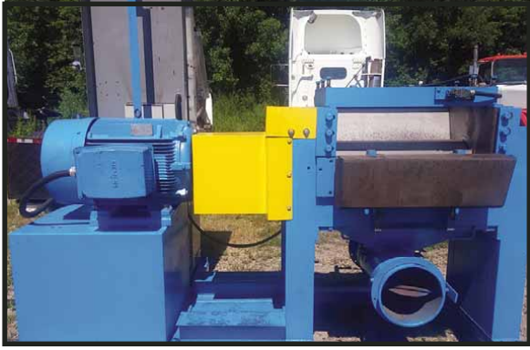
CUMBERLAND MODEL 30 TIRE GRANULATOR Recently rebuilt, 100 hp.
