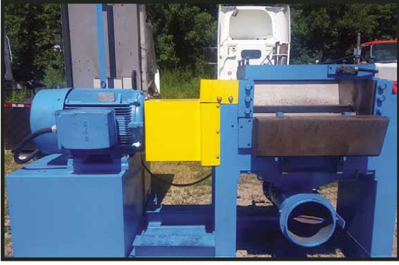
CUMBERLAND MODEL 30 TIRE GRANULATOR Recently rebuilt, 100 hp.
