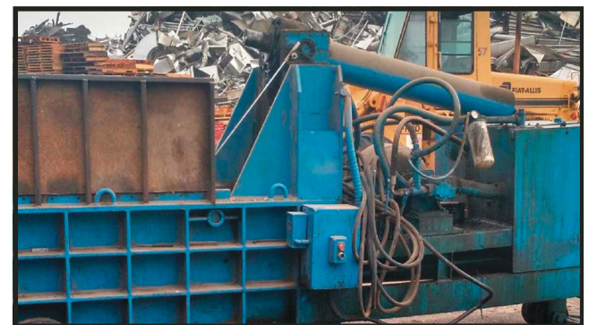
Mosley Portable Tin Baler 24" x 32" bales. 40 HP motor.
