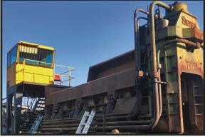
SIERRA 500T STATIONARY SHEAR Rebuilt cylinders. New knives.
