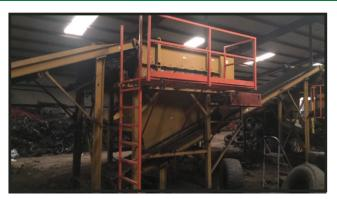
**Granutech Saturn 62 x 40 Tire Shredder** 300 HP motor. Includes conveyance!
