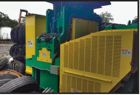
**2011 CM LIBERATOR 2R** Rebuilt and ready to run. The best machine for wire separation and wire free rubber material.
