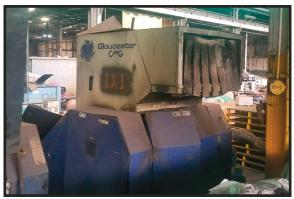
GLOUCESTER GRANULATOR MODEL G1842-5K 48" rotor, 100 HP motor.
