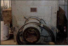
SIEMENS 1500 HP SHREDDER MOTOR 900 rpm, 3-phase, 4,000 volt.
