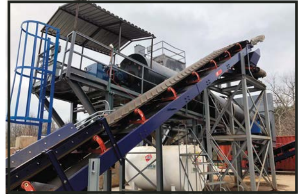
NEWMAN INDUSTRIES COUNTERFLOW DRYER
