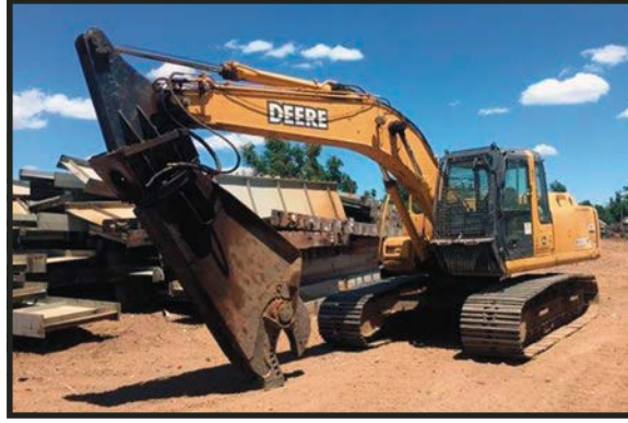
2005 JOHN DEERE 200LC Equipped with a Genesis 300R shear.
