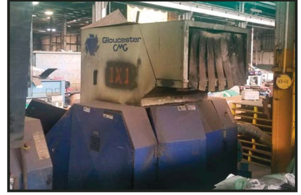
GLOUCESTER GRANULATOR MODEL G1842-5K 48" rotor, 100 HP motor.
