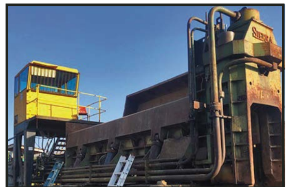
SIERRA 500T STATIONARY SHEAR Rebuilt cylinders. New knives.
