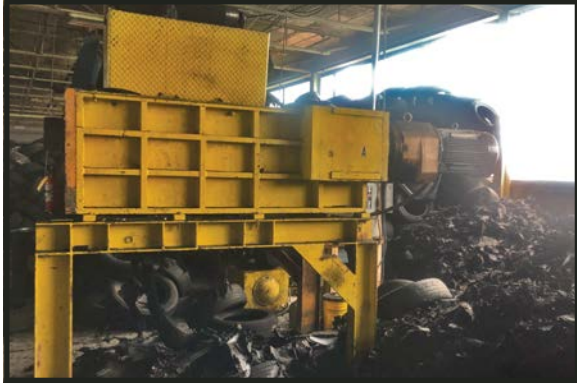
SHRED-TECH ST100 TIRE SHREDDER (2) 50 HP motors. New shafts and bearings.
