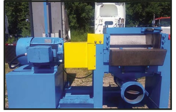
CUMBERLAND MODEL 30 TIRE GRANULATOR Recently rebuilt, 100 hp.
