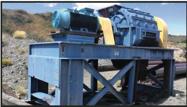
American Pulverizer Ring Mill Model 4800. Recently rebuilt!
